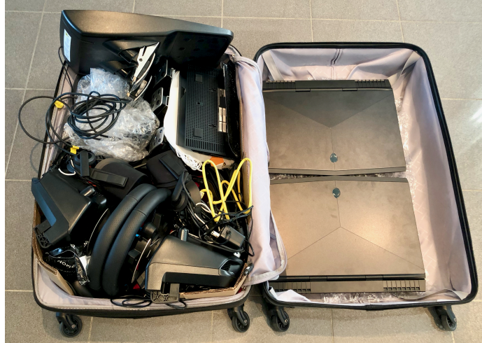
Figure 4.2: The complete StrangeLand simulator hardware in one suitcase (with packing foam removed). The updated version requires even less space and hardware. See Figure 4.3
