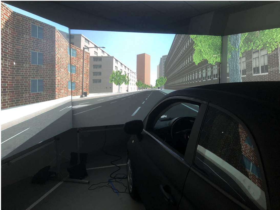
Figure 1.4: Static Driving simulator with vehicle cabin and three projector screens at Cornell Tech NYC. Credit: Wendy Ju.
