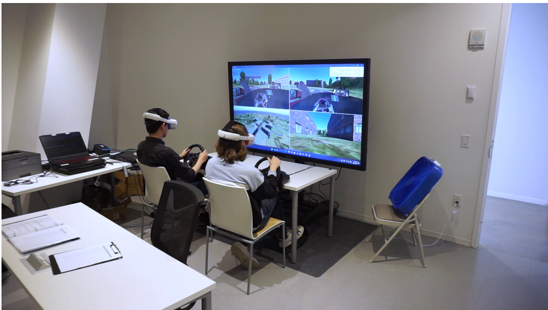
Figure 4.4: Setup of the re-implemented StrangeLand from 2023. The Screen in the back, while helpful for demonstrations, is not required to run the simulator.
