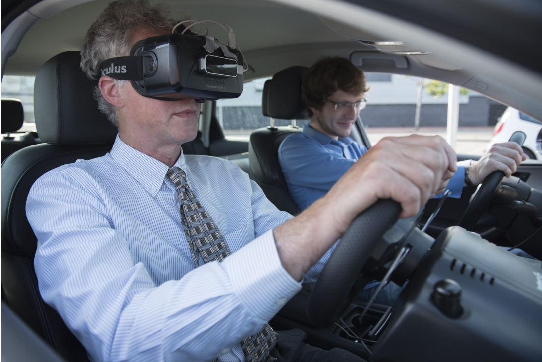
Figure 2.1: VR-OOM allows participants to experience the physical sensations of the real world with controlled virtual environments and events.
