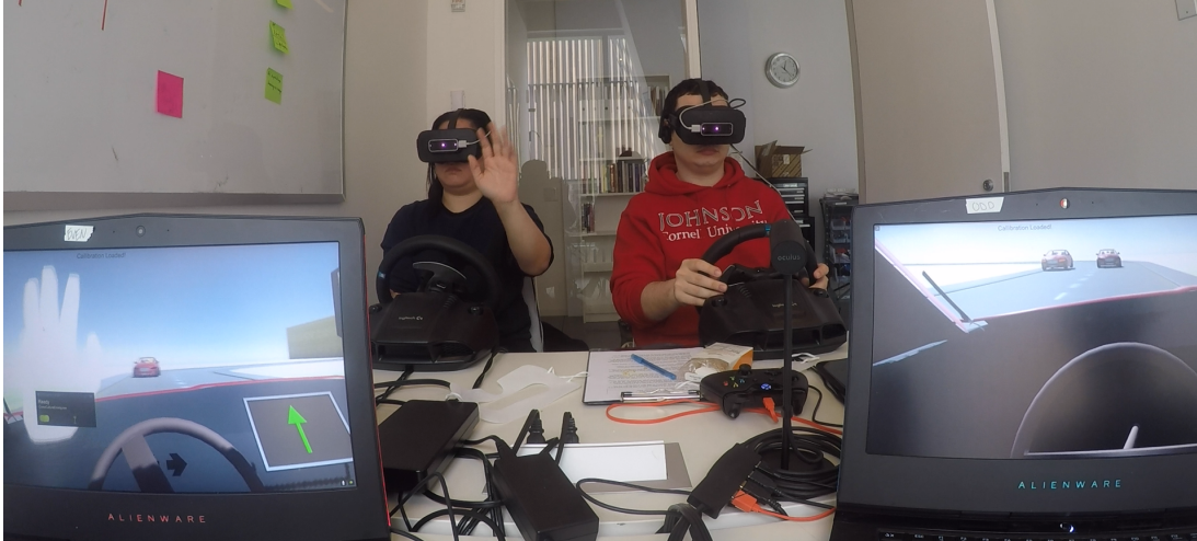
Figure 4.1: StrangeLand uses a multi-person virtual reality driving simulation environment to help illuminate how drivers interact in different cultures. The participants are wearing VR headsets with leap motion (hand-tracking device) mounted on the front. Their hands are on the steering wheels, and gesturing at each other. Across from them are laptops facing the researchers.
