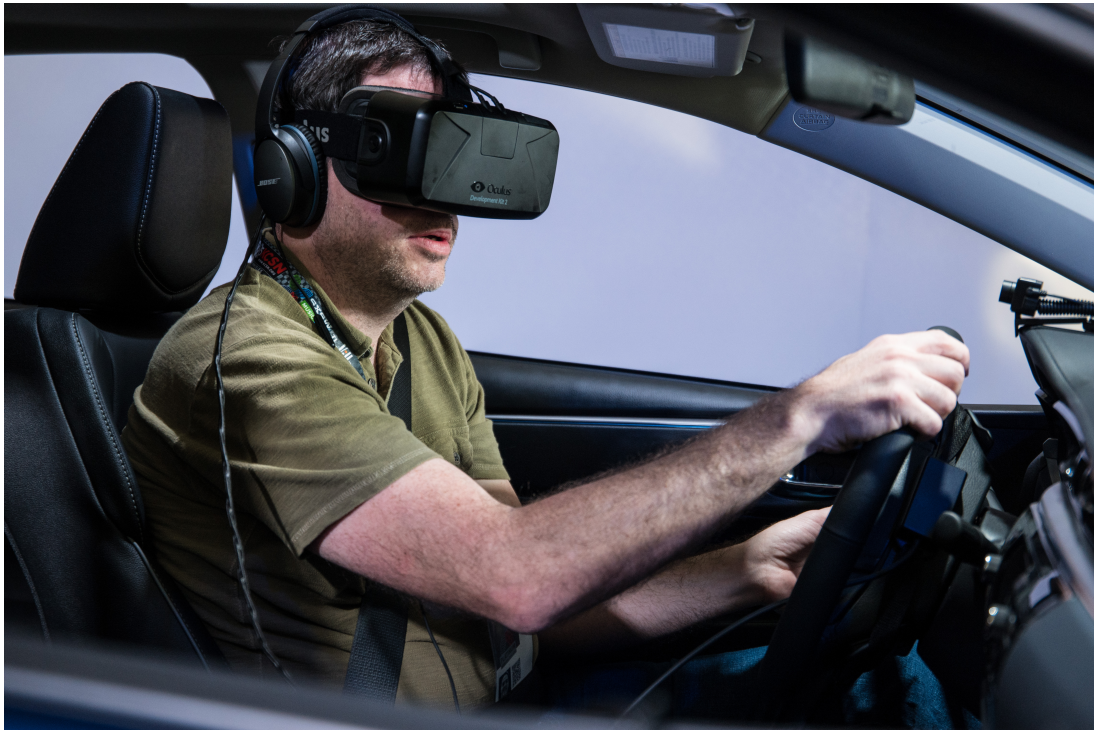
Figure 1.3: Simulator using an Oculus DK2 as the main Display technology. (March 19, 2015) By Nan Palmero from San Antonio, TX, USA. Used under (CC BY 2.0)
