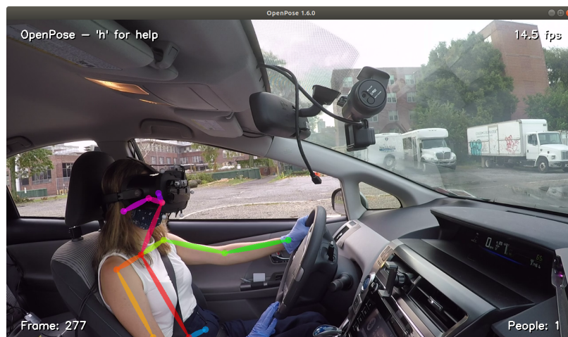
Figure 6.2: Capturing the participant with a regular camera allows us to measure the participant's motion and position.
