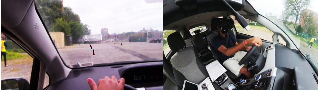
Figure 3.1: XR-OOM enables experimental studies where participants encounter virtual objects (cones) while driving a real car.
