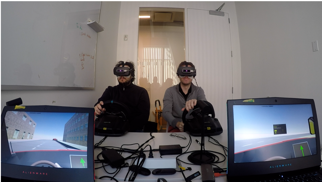
Figure 4.10: We used video recordings with the participants' screen captures in view to validate both the motion-to-photon delay and the network synchronization delay.
